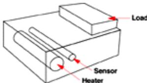
We call a system "static" when there is slow thermal response from the heat source, slow heat transfer, and minimal changes in the work load. When the system is static, placing the sensor closer to the heat source will keep the heat
