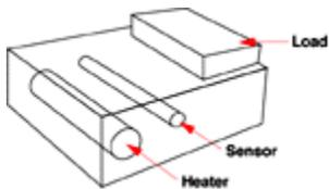
When the heat demand fluctuates and creates a system between static and dynamic, place the sensor half-way between the heat source and work load to divide the heat transfer lag times equally. Because the system can produce some overshoot and/or undershoot, we recommend that the electronic controller selected for this situation include the PID features (anticipation and offset ability) to compensate for these conditions. This sensor location is most practical in the majority of thermal systems.
